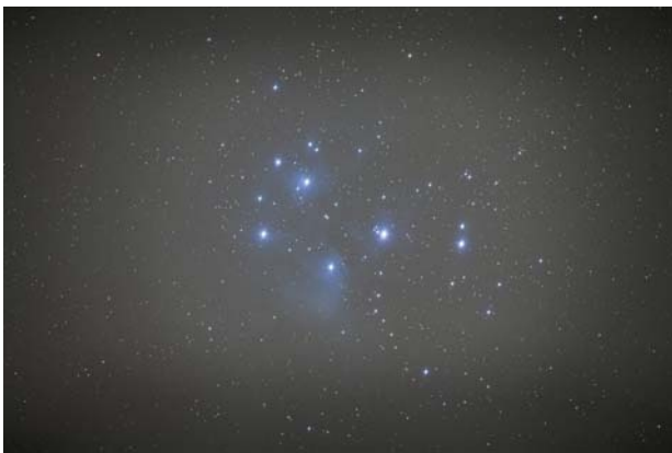
An unprocessed raw image recorded with a Canon EOS 5D Mark II full-frame DSLR displays the level of vignetting introduced mostly by shadowing from the camera adapters and DSLR's mirror box. Note that the image is also flipped mirror-image.
