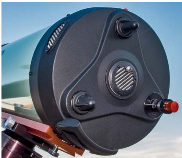
The back cell includes the dual-speed Feather Touch focuser, fan vents for cooling the tube (and battery pack input), and two knobs for locking down the mirror once it is focused.
